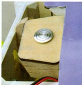
I glued on a simple wood bracket to the firewall and mounted the F1 fueling system from Slimline to it. I have an identical one mounted on the bottom of the plane for the overflow line.
