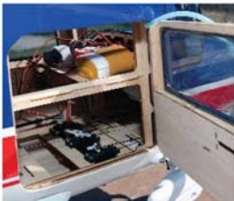
The large cabin door makes access easy for all the radio gear. Note that due to the shelf above the servos you will need a short screwdriver to install them.
