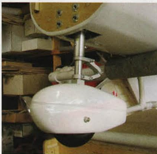
The Cessna 150 ARF kit includes a nicely done scale front wheel. It's mounted inside the fuselage, so be sure to lock down everything tightly.
