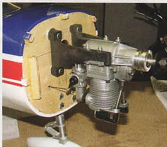
The Saito 1.80 has plenty of room under the cowl for good airflow and easy firewall mounting. The engine provides outstanding performance and pulls the Cessna around with good authority.
