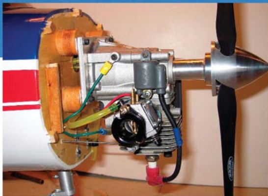
The Zenoah G-26 is a great power plant for this airframe, well known for its reliable power and easy handling.
