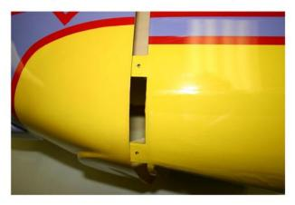
Make some cardboard guides to mark and drill holes to accept the small cap screws, (provided) and bolt the cowl into place temporarily.
