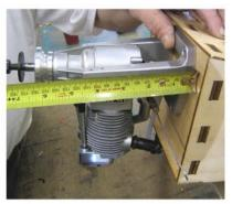
The firewall has some right thrust built in. You may want to add up to 3 degrees of down thrust
