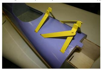
You may have to bend the ends to match the angle of the top wing center rib that these get bolted to. When you are satisfied with the alignment, tighten all screws.
