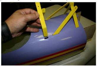
Insert the pre bent center cabane brackets into the slots. Be careful to align the holes and attach with supplied cap screws to the "T" nuts that are pre-installed inside the fuselage. There are 2 vertical pairs and one pair at 45 degrees which attach midway on the front vertical parts.
