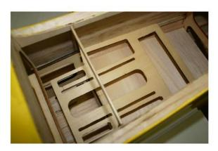
Be careful not to break the tray by over-bending. Once in place, glue permanently in place with C/A glue.
