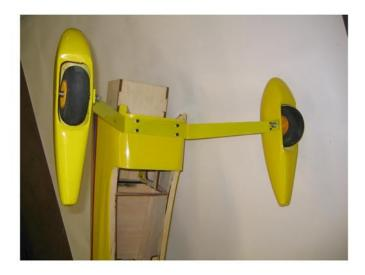
We have included a pair of triangular "Spat"s that can be attached to the outside of the landing gear on both sides to give the airplane even more scale detail.
