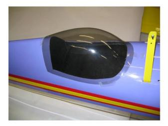
Your canopy is pretrimmed and ready to be installed on the fuse. Position the canopy over the cutout area in the fuse. Use pieces of tape to hold it in place. Mark 3 places for the screws along the lower edge on both sides of the canopy. Drill holes on the marks using a 1/16 dia. bit. Reposition the canopy over the fuse making sure it is even on both sides of the fuse.
