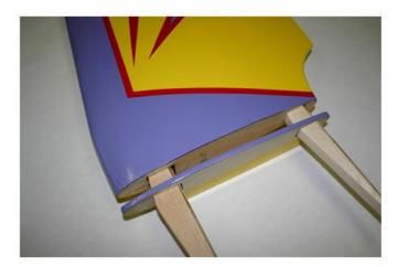
If needed, slightly sand the wing roots to assure a tight fit.
