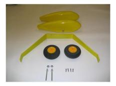
Set the fuse on its wheels and mark the location of the wheel pants, assuring the proper angle to the surface.
