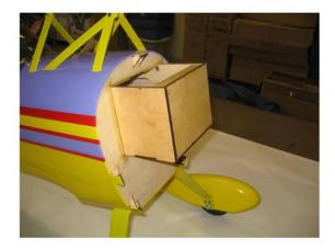
Temporarily fit the engine in your motor mount and position on the fuselage. Then temporarily fit the cowl on the fuselage and locate the engine mount so the prop shaft exits the center of the cowl opens. Mark the location of the cowl with masking tape. Gently lift off the cowl and mark the location of the engine mount.
