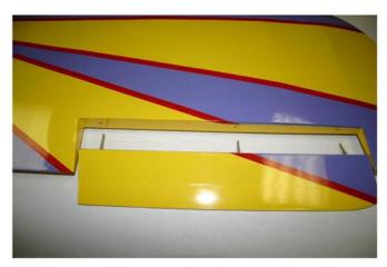
Install the aileron hinges with epoxy, allowing no gap. Repeat the process for both wings
