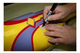
You can use a similar guide to mark the location where the needle valve extension will come through the top of the cowl. Mark and drill this location. Also mark and drill the location where the fuel dot will be installed.
