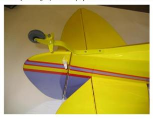
On the bottom of the rudder a slot is cut with a razor saw approximately 3/4" up from the bottom 5/8" deep to the metal double sided control horn. Carefully center the control horn in the slot and epoxy glue into place. Install control spring.
