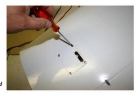
Note: Installation of optional control surface corrugations: If you opt to install the corrugations on control surfaces (ie ailerons, flaps, etc) cut away the covering, leaving an edge of 1/8" all around of the corrugated piece being installed.
