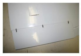
Make sure all the hinges are aligned and are tight to the wing surfaces.
