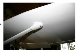
When satisfied with the fit use silicon sealant or hot glue to secure the cuffs to the ends of the strut. Make sure the cuffs do not protrude past the aluminum of the strut ends.
