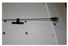
Position the trumpet style control horns at the leading edge of each aileron with the clevis and rod installed along side the aileron servo horn.
