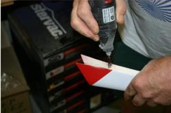
Place the fin extension over the fin and center it on the fuselage top. Use a dremel tool to trim the notch on the bottom of the extension to assure a tight fit against the fin.
