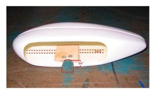
You will notice a groove in the plywood for the ridge in the wheel pant as shown in photo.
