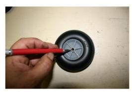
Using an Xacto, clean out around the main gear wheels to ensure a nice free fit on the axels.
