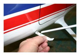
Using a sharp Xacto knife, remove the covering from the Fuselage where the Wing Strut Tab will be located. Look inside the Fuselage to see where the Wing Strut Tab gets bolted and make sure you cut the hole in line with this.
