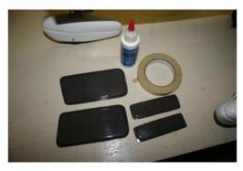
Use canopy glue (RC-56 or similar) to secure the precut windows in their positions. They are glued along the inside edge. Trim to fit opening.
