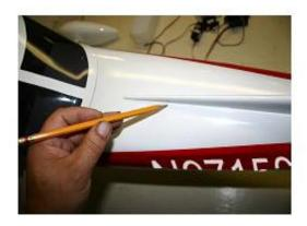
Remove the fin extension and using an Xacto carefully cut just inside the pencil marks.
