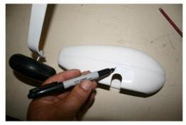
When the glue is set, temporarily mount the wheel pants over the axels, making sure they are level with the fuselage. Mark through the predrilled holes onto the wheel pants.
