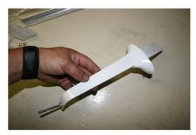
Bolt the main gear axels to the legs and slide the gear cuffs over the ends of the legs.
