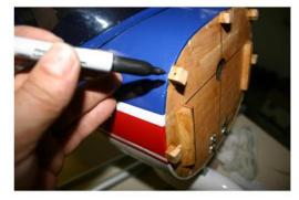
Position the cowl under the papers making sure the painted lines on the cowl are all even and aligned with the covering lines on the fuse.
