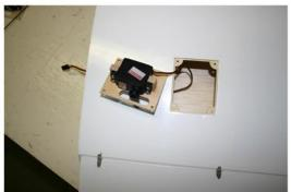
Using Epoxy glue (or similar) install all hinge points into the pre-drilled holes. Make sure not to get excess glue on the hinge pins. Remove excess glue with alcohol and paper towel.
