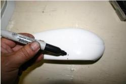
Rough up the inside surface of the wheel pants with sand paper, making sure they are right and left pair. Wipe off the dust and clean the area.
