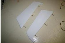
Glue the elevators into the stabilizer. Wipe off any excess glue. You may have to drill holes in the elevators for the joiners.
