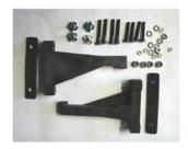
Install your engine so the distance from the wire wall to the back of your propeller is  $6\frac{1}{2}$  inches. We recommend positioning your engine with  $3^{\circ}$  of down thrust and  $2^{\circ}$  of right thrust. Use flat washers if needed.
