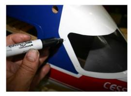
Locate the rear windshield and center it on the fuselage keeping it tight against the fuse.
