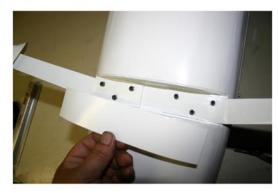
Place the factory FRP main gear cover over the gear. You will notice it fits into the ledges along the fuse. Trim to fit the ledges and landing gear.
