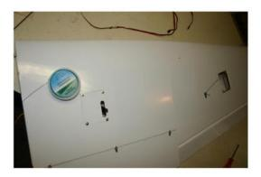
Note: You will notice the flap servos are mounted so they both travel in the same direction unlike the ailerons, which are mounted on opposite sides of the servo bays so they can travel in opposite directions.
