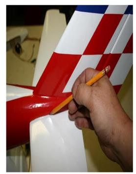
Push the stabilizer through the fuse and center it using the marks. You may need to sand slightly to fit. Using a pencil, lightly mark the stabilizer along the fuse sides top and bottom. Remove it and carefully cut 1/8" inside the line using a sharp X-Acto to remove the covering. Just cut the covering, not the balsa underneath.
