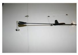
When you are satisfied with the fit and position of all controls, makes a Z bend on the servo arm end of the control rod.
