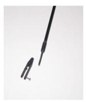
Mounting the elevator control horn is very similar to the rudder but uses a push rod assembly.
