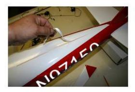
Tip: Rubbing Alcohol works great for cleaning off excess epoxy
